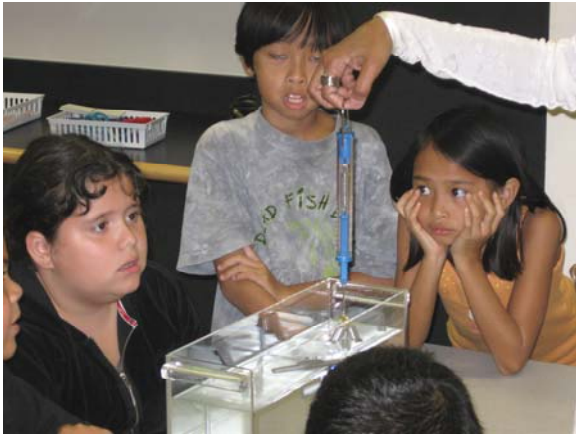
Observing the concept of buoyancy, demonstrated by dunking weights suspended by a spring scale into water
